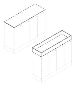
These surfaces are to be placed on top of the lockers and to cover the top of the corner cabinet to allow better uniformity.
