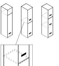
There is one ventilation grille per level with the lockers with doors. The back is split where the shelf is positioned and the shelf is visible on the back, but not the sides.
