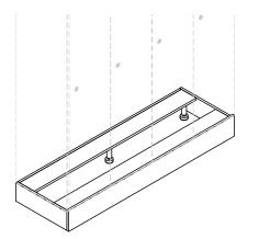
The platform is necessary to support the lockers. Its front is removable and an opening provides access to adjust the levelers. The platforms do not require any assembly on delivery other than the levelers.
