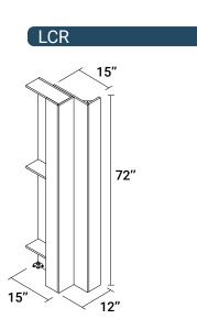
Corner unit: · Delivered disassembled; 5/8" laminate; · White nylon levelers. Restriction : Only available for 72"H lockers. Application : The corner unit covers the height of the platform and the lockers. It allows a nice finish between lockers installed at 90°. It is composed of 2 modules, the first of fixed width (7") and the second of adjustable width (0-6'). The adjustable module is on the right for the LCR item, and on the left for the LCL item. See appendix
