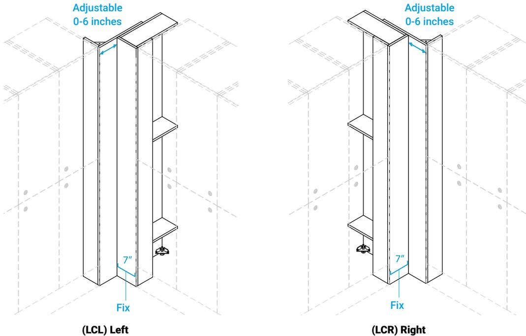
The corner unit allows a nice finish between the lockers installed at 90°. It is composed of 2 modules, the first of fixed width (7") and the second of adjustable width (up to 6"). The adjustable module is on the right for the LCR item, and on the left for the LCL item. It covers the height of the platform and the lockers. Available only for 72"H lockers.
