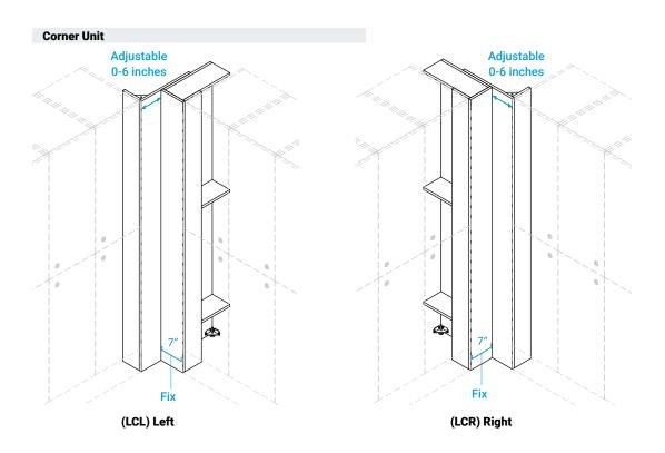
The corner unit allows a nice finish between the lockers installed at 90°. It is composed of 2 modules, the first of fixed width (7") and the second of adjustable width (up to 6"). The adjustable module is on the right for the LCR item, and on the left for the LCL item. It covers the height of the platform and the lockers.
