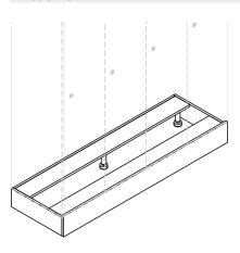
The platform is necessary to support the lockers. Its front is removable and an opening provides access to adjust the levelers. The platforms do not require any assembly on delivery other than the levelers.
