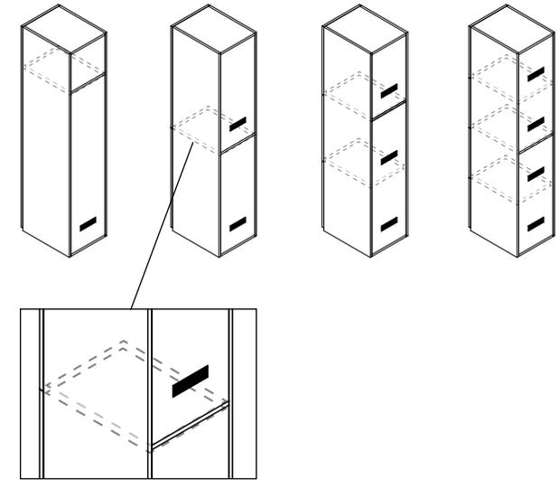
There is one ventilation grille per level with the lockers with doors. The back is split where the shelf is positioned and the shelf is visible on the back, but not the sides.
