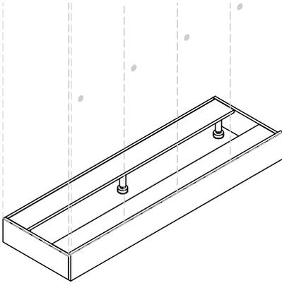
The platform is necessary to support the lockers. Its front is removable and an opening provides access to adjust the levelers. The platforms do not require any assembly on delivery other than the levelers.
